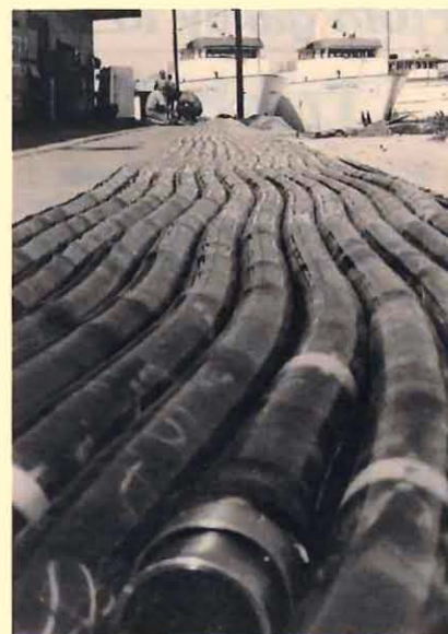
Streamer sections on Galveston dock.
