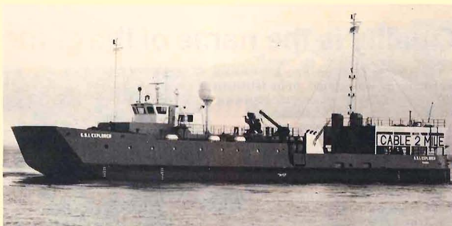
M/V GSI Explorer uses Hull originally intended for transport ferry.
