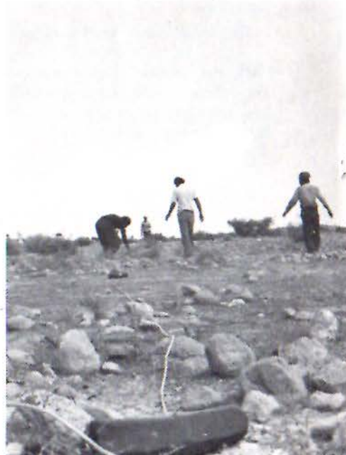
Shooting crew laying out the explosive cord with the dynamite set on top.
